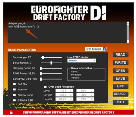
3 Plug in servo, click "Read" button to read servo parameter to current interface (as pic).
